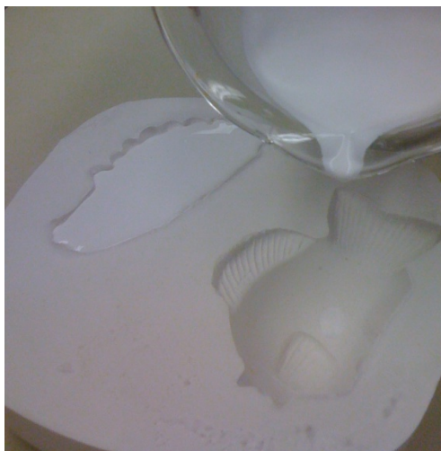
Figure 4: Pouring ceramic slurry into a plaster mold
