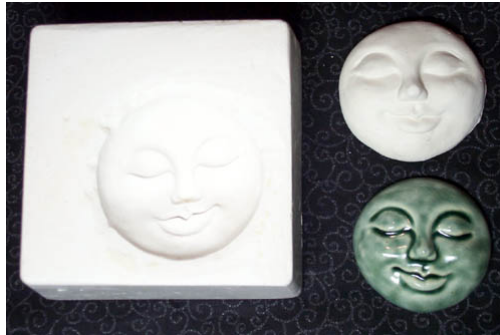
Figure 3: Plaster mold with model and final cast piece ** wetcanvas.com
