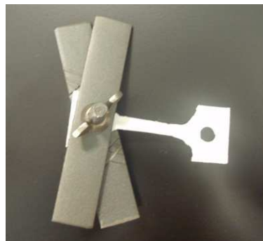
Figure 4: (a) Strike plates with a specimen (b) fractured specimen
