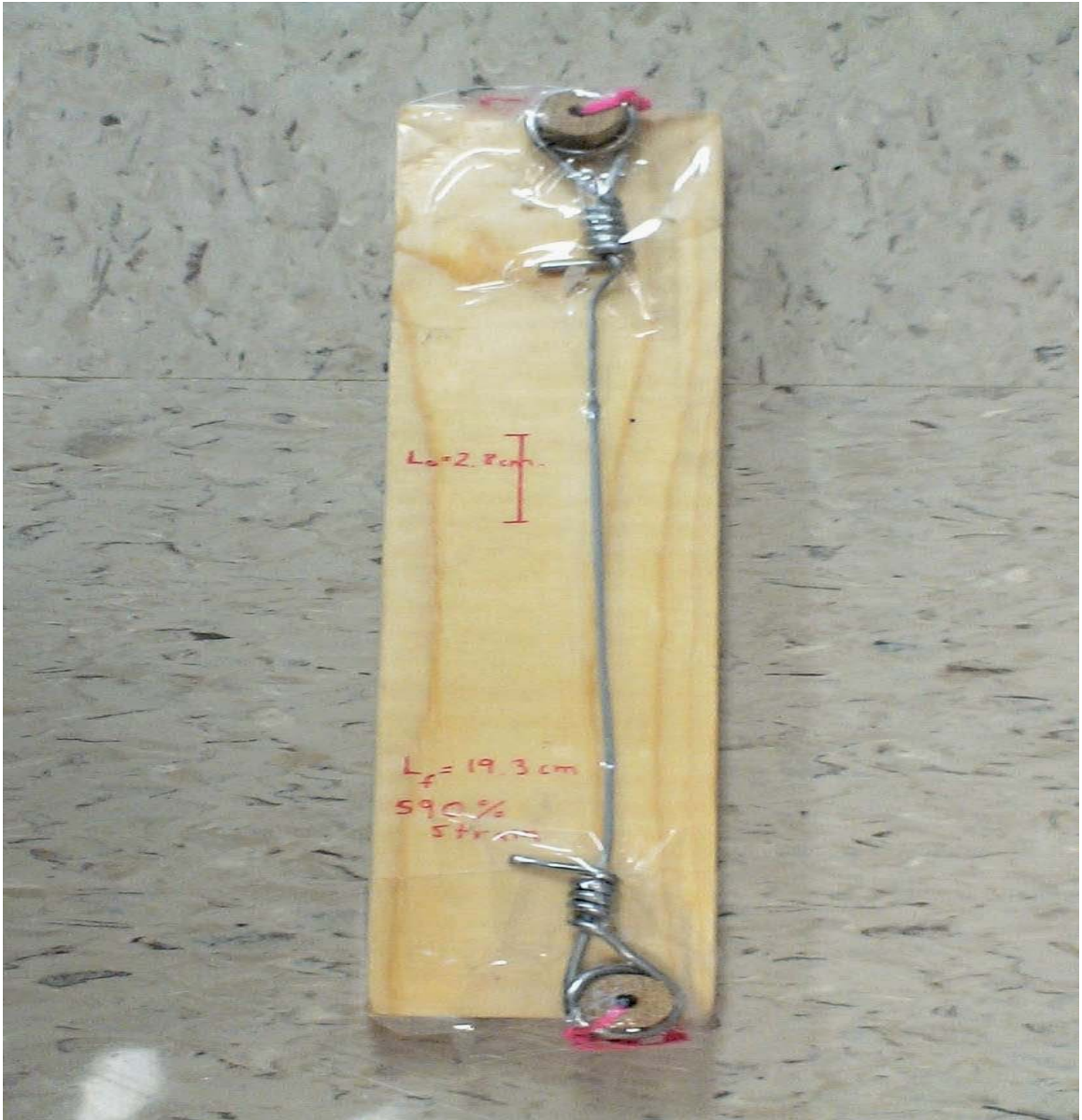
Figure 2. Highest-Strain Specimen Tested to Date; Strain is Almost 600%.
