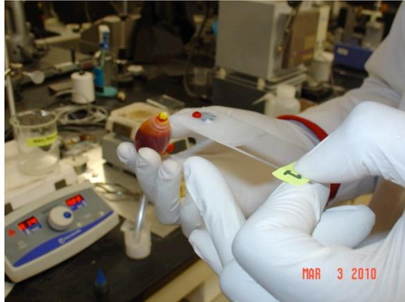
**Figure 4: Place one drop of red dye (food color) in the center of the wax attachment, directly on top of previous blue dye location.**
