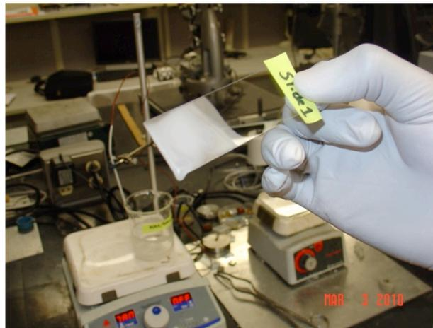
**Figure 2: Glass slide (1) dipped 4 times in a wax beaker**
