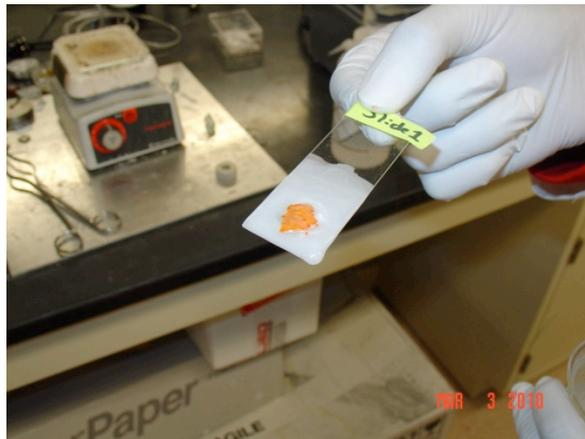
**Figure 5: Slide with multilayer controlled release coating**
