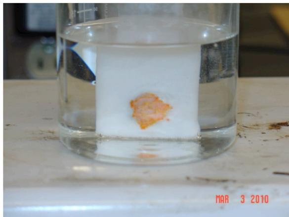
**Figure 6: Slide with multilayer colored coating in vinegar beaker (Prior to release)**
