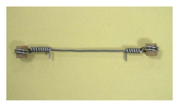
Figure 1. Solder Creep Specimen Ready for Use.
