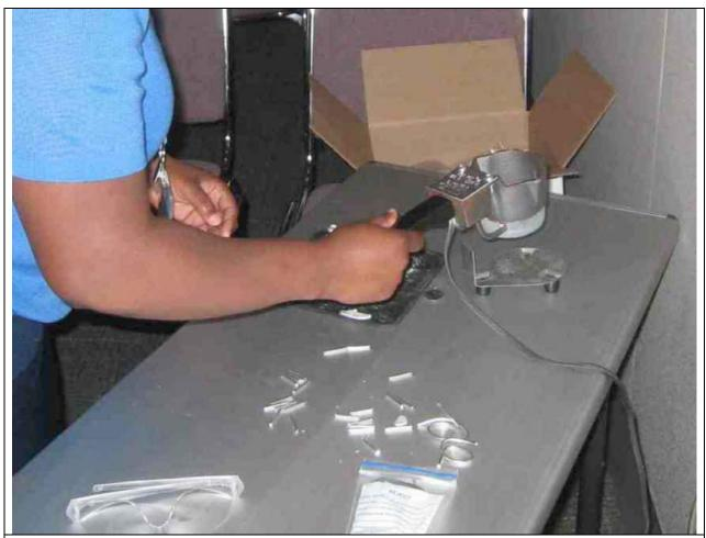
Figure 2: Pouring solder into a mold.
